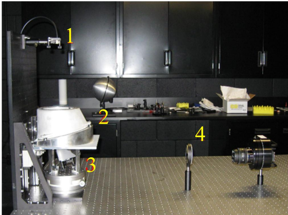
Figure 2: Picture of the grating alignment assembly with features indicated as follows: (1) Fiber head (note that the collimator lens is not seen in this photo). (2) Grating cell holding grating substrate mounted on alignment bracket. (3) Rotary stage. (4) Focusing mirror and CCD.
