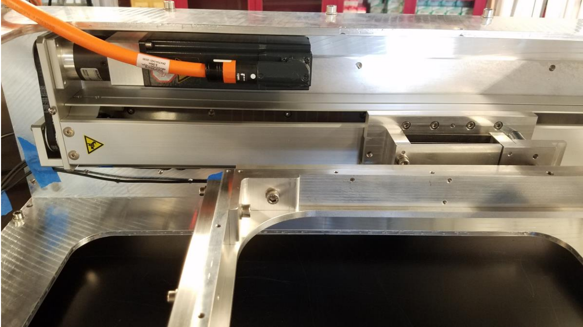
Figure 12. The Beckhoff motor and the THK rail cart.
