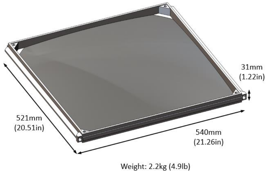
Figure 5. Concept of the GMACS slit mask in its cartridge.
