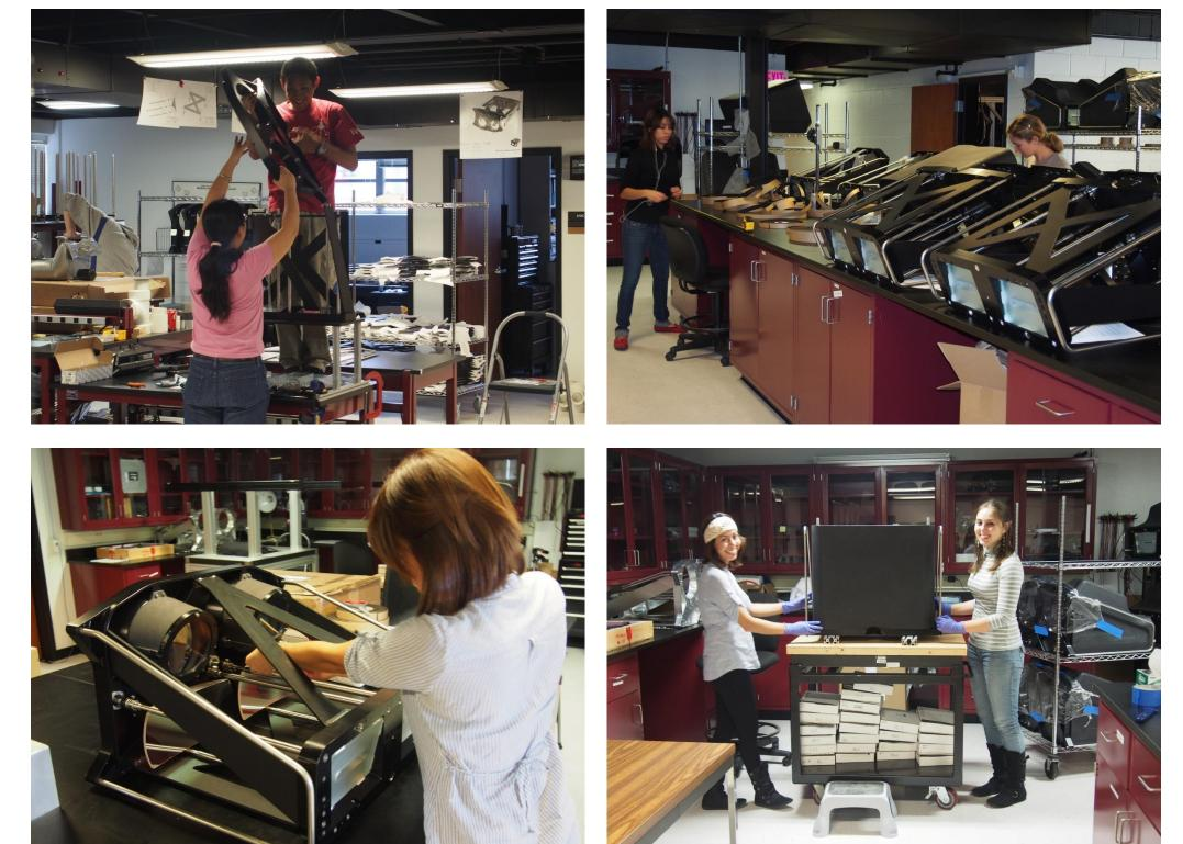
In the end, the final mating of collimator subassemblies into a complete collimator unit was accomplished relatively quickly, with the final thirty pairs of collimators being assembled in just over two weeks in December 2013. The record assembly time of fifteen minutes to complete one pair of collimators is shared by the team of Nagasawa and Li.
