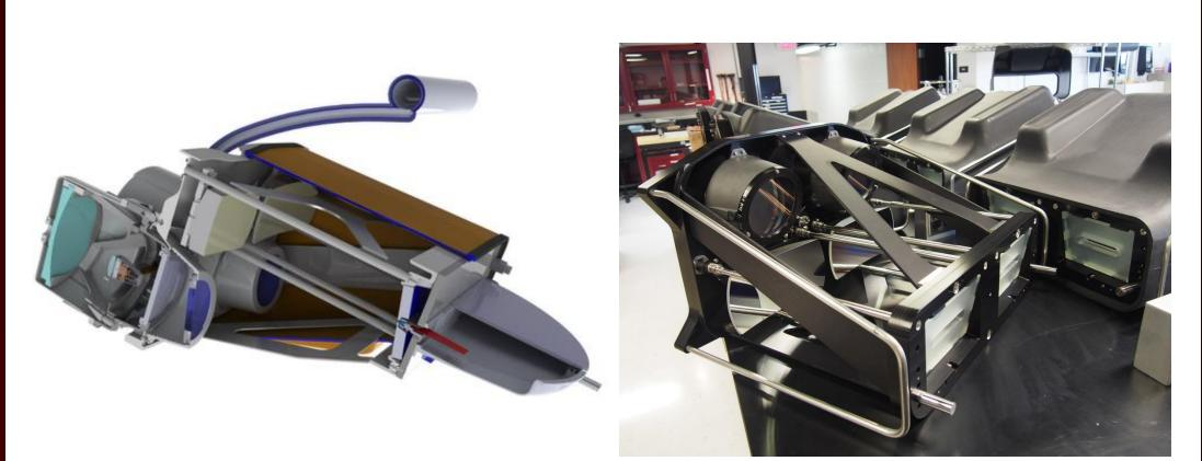
Left: Section-view drawing of a pair of VIRUS spectrographs. Right: One complete collimator with all optics installed. Additional completed collimators (with their protective covers installed) may be seen in the background
