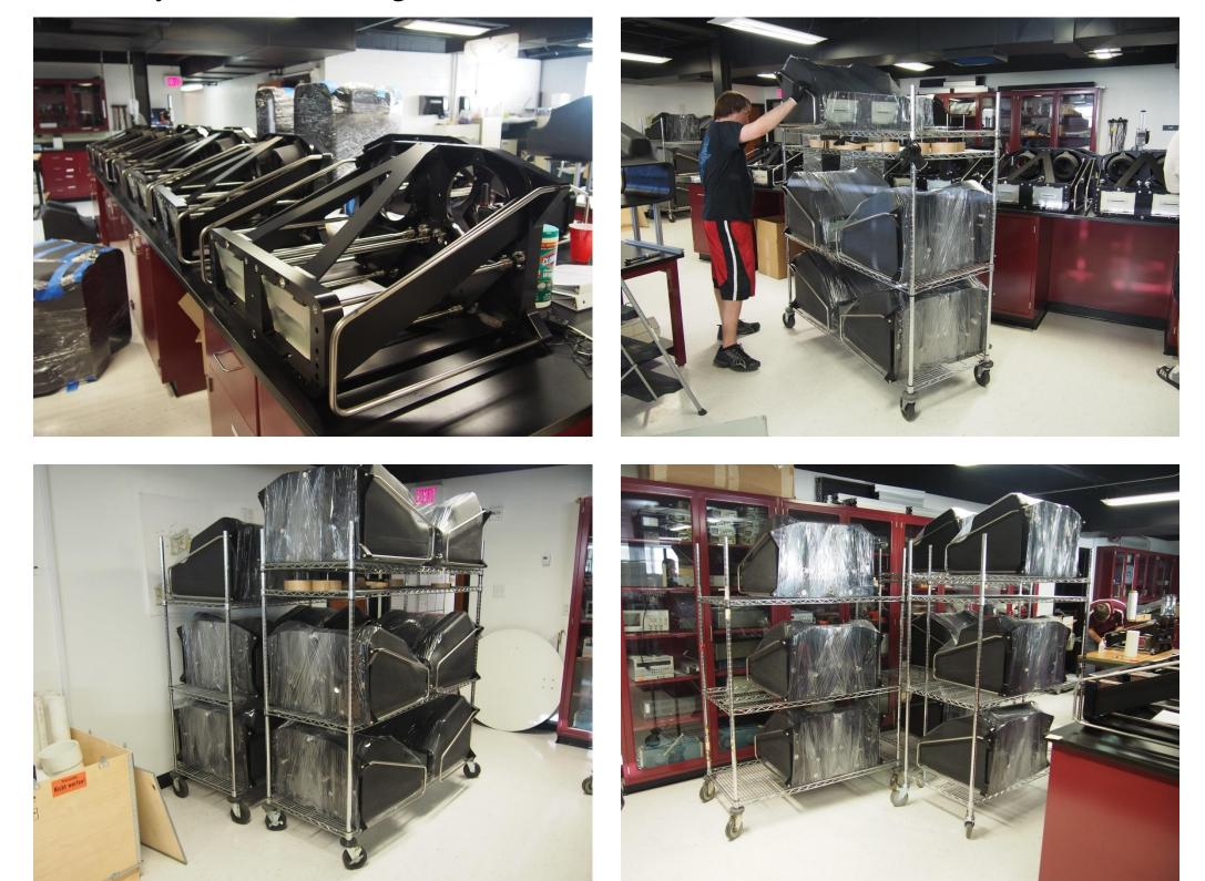
Once the final collimator assembly is complete no further optical alignment is required at this stage. The completed collimators are fitted with a plastic cover that remains with the collimators once installed on the telescope, protected from dust with plastic wrap, and finally packaged and shipped to UT-Austin for integration with the VIRUS cameras and final optical alignment.
