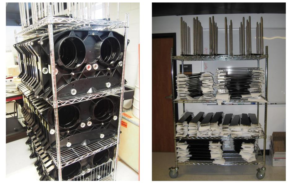
Collimator subassemblies were pre-assembled and stored before the final collimator assembly. Shown here are the base plates (left) and side, top, and bottom plates (right). Each of these components has multiple alignment and attachment features to facilitate the final assembly. Collimator mounting plates with attached Invar metering rods can be seen on the top rack of the carts.
