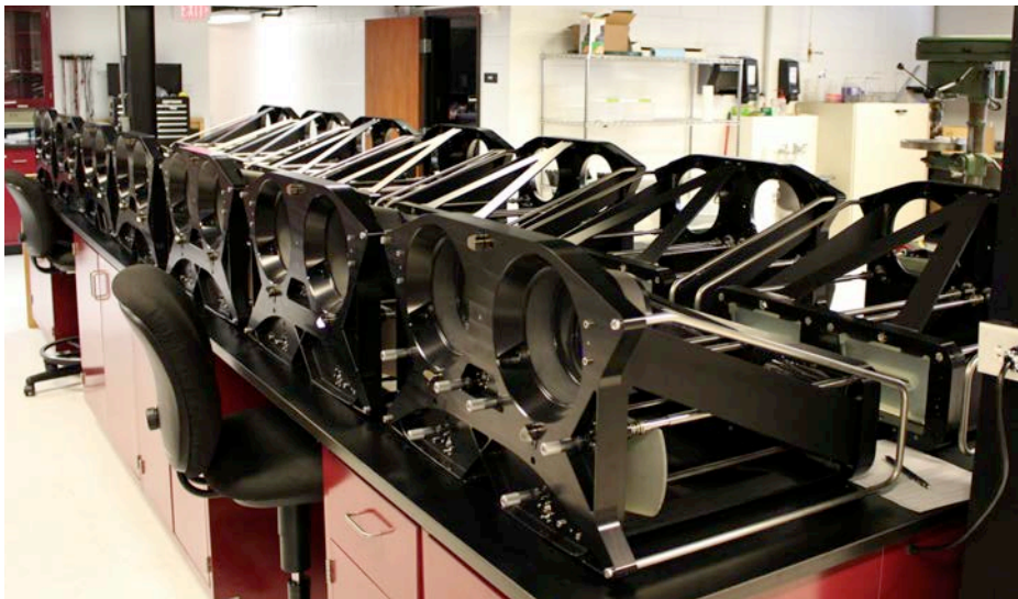
Figure 5. Twelve completed collimators arrayed on the assembly line at TAMU
