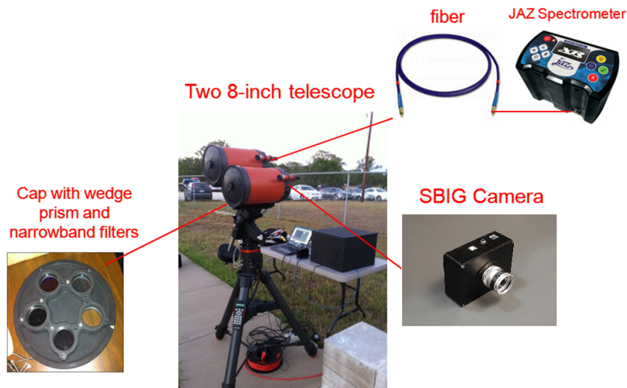
Figure 6. Setup of the aTmCam prototype.
