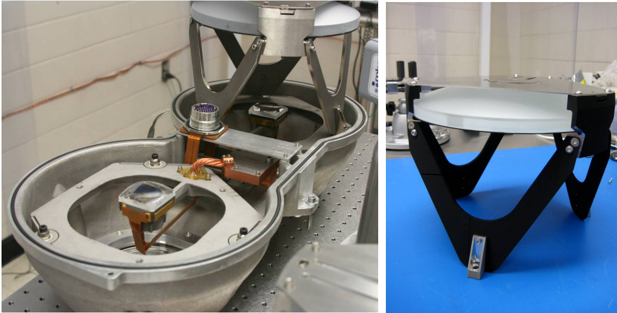
Figure 5. Production camera assembly and alignment. Integration of the CCDs and field flattener lenses into the cryostat is shown on the left. Integration of the camera mirror assembly is shown on the right.
