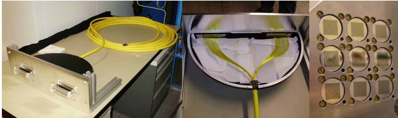
Figure 7. Production IFU cables at AIP. Left and middle images show the slit assembly with the two slit blocks that feed the pair of spectrographs within a VIRUS unit. The slit assembly mounts to the collimator kinematically. The cable length is 22 m. Right shows nine IFUs input heads mounted as they will be at the HET focus. Three screws and a pin locate the heads. AR coated cover plates are not yet applied in this view. The heads have a \frac{1}{4} fill-factor in the field of view. This configuration provides the ability to fill in the field of view by offsetting the telescope to four positions.
