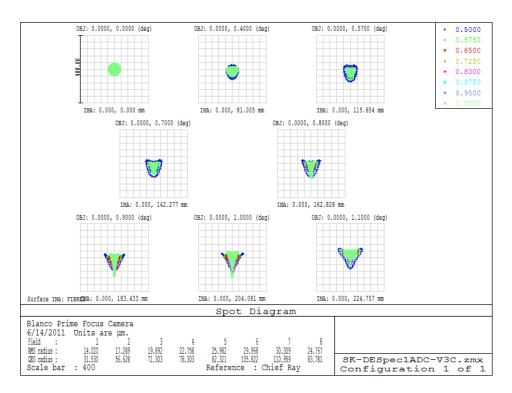
**Figure 2:** The spot size versus wavelength (0.5 (blue)–1.05 (green) microns) from the center of the focal surface (top-left) to the edge of the focal surface (radius of 1.1 deg, lower-right). The RMS spot radius is 0.26 arcsec at the center, 0.52 arcsec at the worst radius, and 0.44 arcsec at the edge. These results are from the "DESpec-SK-3C" design.
