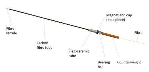
**Figure 6:** The MOHAWK unit fiber positioner. The spines pivot from mounts at the base and are driven by piezo-electric actuators.
