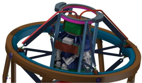
**Figure 7:** A schematic drawing of a MOHAWK-style fiber positioner positioned on top of the DESpec corrector optics, including the fiber bundles that would feed potential DESpec spectrographs.
