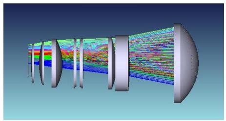
**Figure 1:** One option (DESpec-SK-3C) for the DESpec optics. From right to left they are C1 to C3, the two-component ADC, C4, C5', and the field-flattener C6. The focal plane of fiber-ends would be just to the left of the new C6. "C1" is a little less than 1 meter in diameter. The optical train is 1.9 meters long. C1, C2, C3, and C4 are already installed on the telescope as part of DECam.
