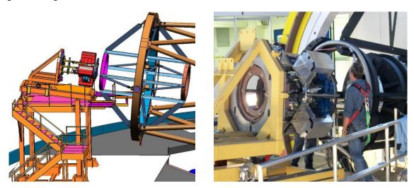
**Figure 11:** The DECam camera installation fixture (schematic at left, in close-up at right) at Fermilab. Right image shows the installation fixture being used to mount the camera in the Prime Focus Cage (black, at right).
