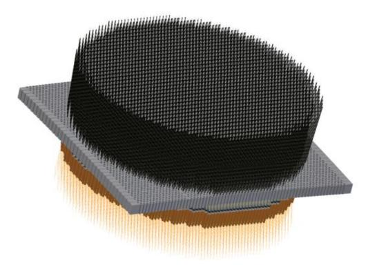
**Figure 5:** The MOHAWK fiber positioner with DESpec specifications, i.e., 4000 fibers with a 7mm pitch, placed in a 450mm diameter focal plane.
