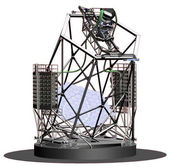
**Figure 1:** The 96 VIRUS spectrograph pairs will be mounted inside two climate-controlled enclosures located several meters above the base of the telescope.
