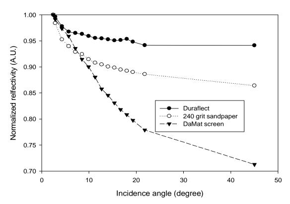
Figure 4. Normalized reflectivity at normal exit angle vs incident angle. Details of the various results are given in the text.
