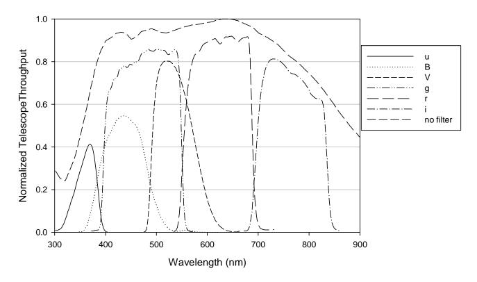
Figure 6. Swope Telescope Throughput
