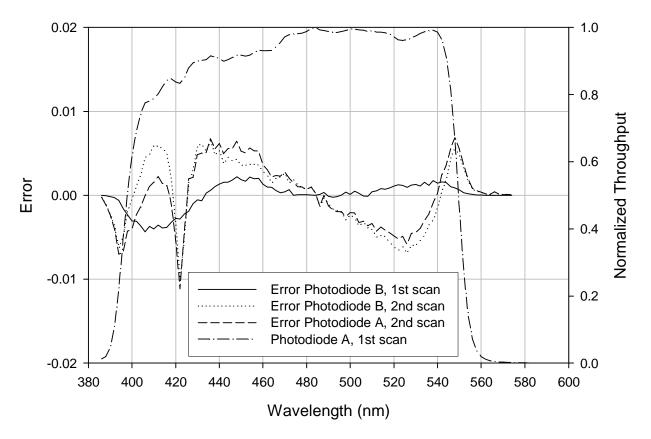
Figure 7. Repeatability of the g filter throughput for 2 separate scans. Error compared to Photodiode A and 1st scan
