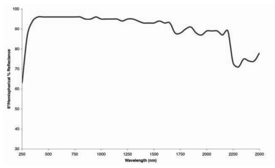
Figure 5. Duraflect reflectivity vs wavelength
