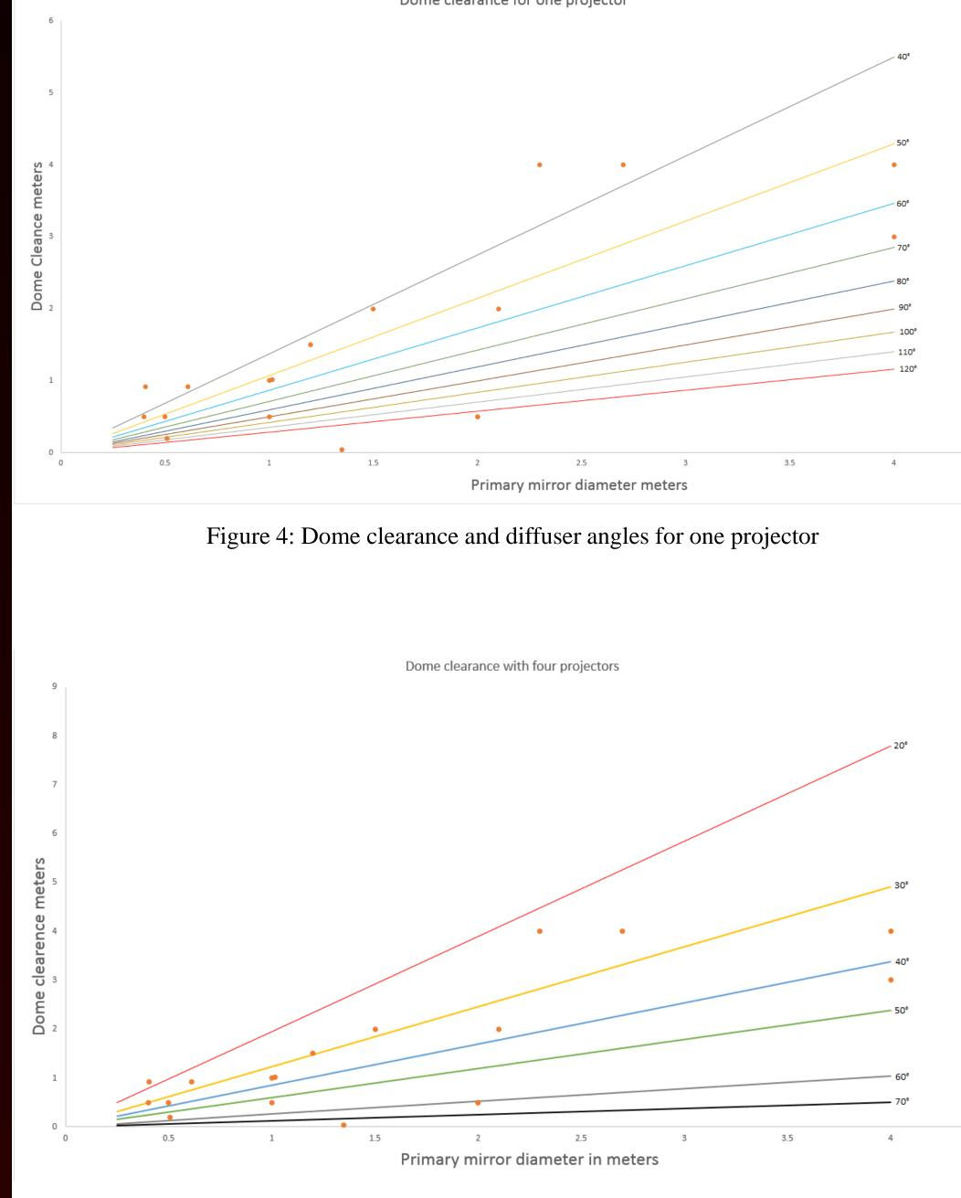
Figure 5: Dome clearance and diffuser angles for four projectors
