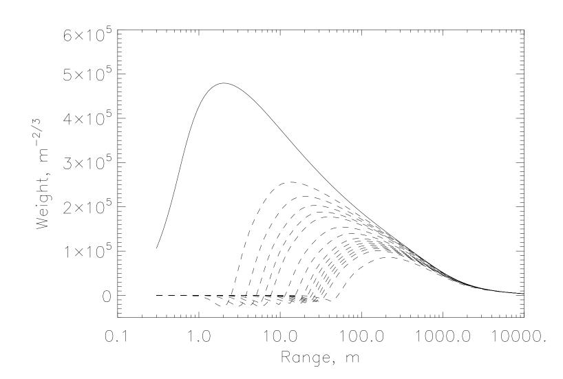
Example of the weighting function. The solid line is a single detector. Greater detector spacing probes higher peak atmospheric ranges.
