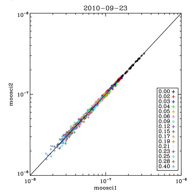
As a further test, MooSci was compared to LuSci which was operated in previous site characterization campaigns successfully. The seeing calculated from the measurements of both instruments agree well with a general offset. MooSci tends to measure a higher seeing as compared to LuSci.
