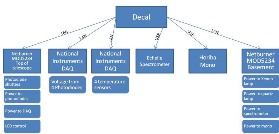
The NetBurner modules are able to use both a TTL signal used for power switches, and analogue signal used to adjust the output of the LEDs.
