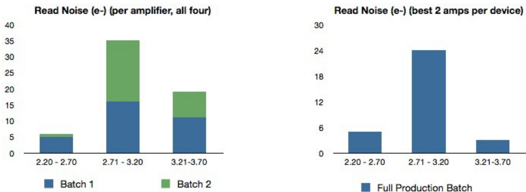
Figure 10. Here we show the read noise for the first production batch of 16 devices. Each device has four amplifiers, for which the read noise has been measured separately. The value for each amplifier is shown in the histogram on the left side (64 total). On the right the best two amplifiers have been selected and plotted. The default is read the upper left and lower right amplifier, but if there is significant deviance of a high read noise amplifier, an alternative amp will be employed. All delivered devices fall below the requirement of less than 4.2 electrons, although this requirement is held over any combination of detector and controller combinations which has not yet been measured.
