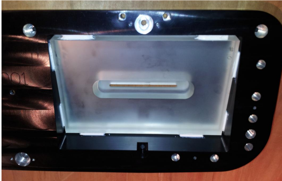
Figure 5. Fold flat mirror glued into an anodized head plate.
