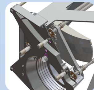
Section-view showing the collimator mirror, mounting plate and micrometers.
