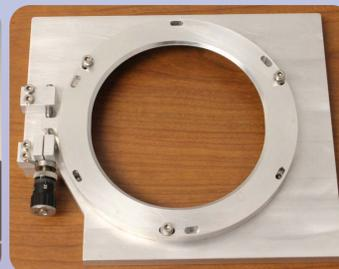
Working prototype of the adjustable grating cell.
