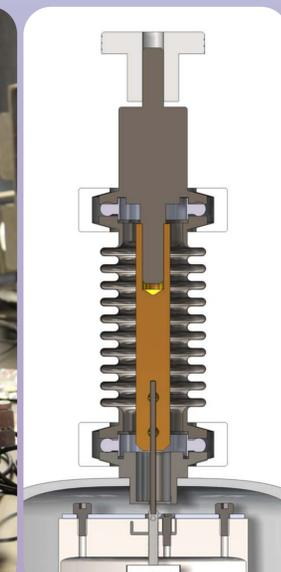
Section view of a ferro-magnetic feedthrough, bellow and hex key tightening a set screw.
