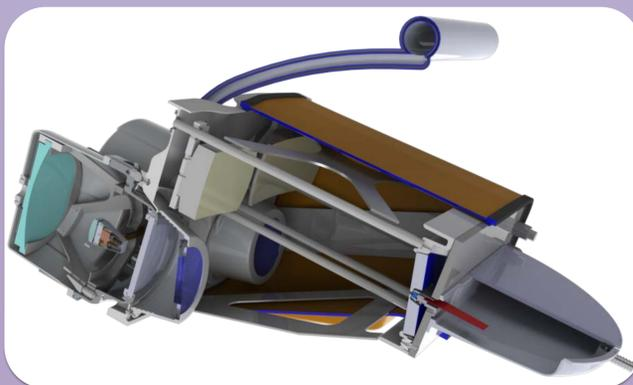
Section-view drawing of a pair of VIRUS spectrographs.
