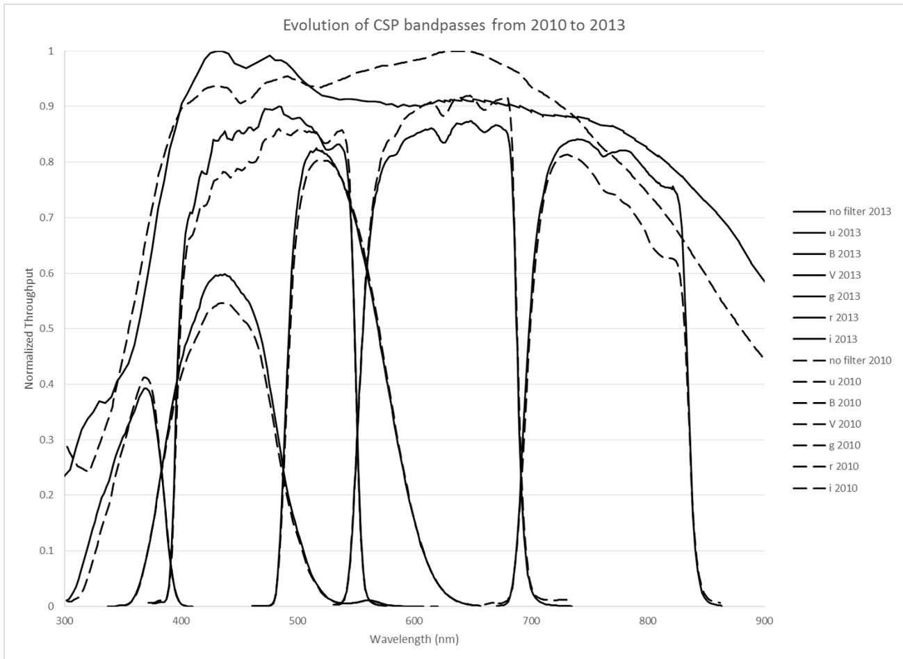
Figure 5: Evolution of CSP bandpasses from 2010 to 2013 for the Swope Telescope.
