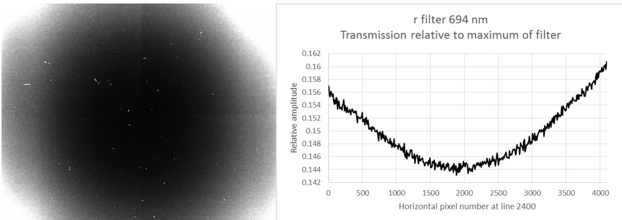
Figure 10a and 10b: (Left) CCD image at 694 nm with r filter, (Right) horizontal slice of the image at line 2400.
