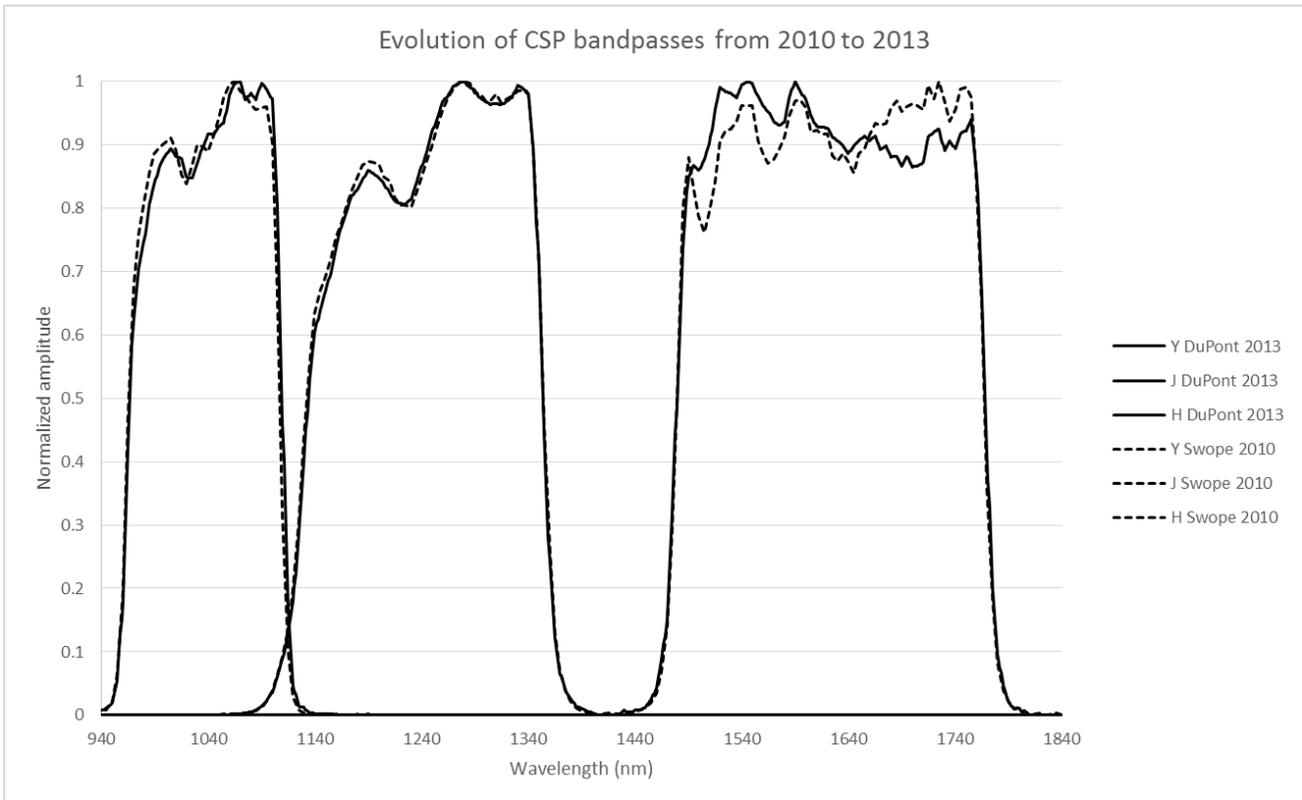
Figure 6: Evolution of CSP bandpasses from 2010 to 2013 for RetroCam
