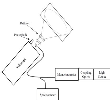
Figure 1. Schematic diagram of TCal
