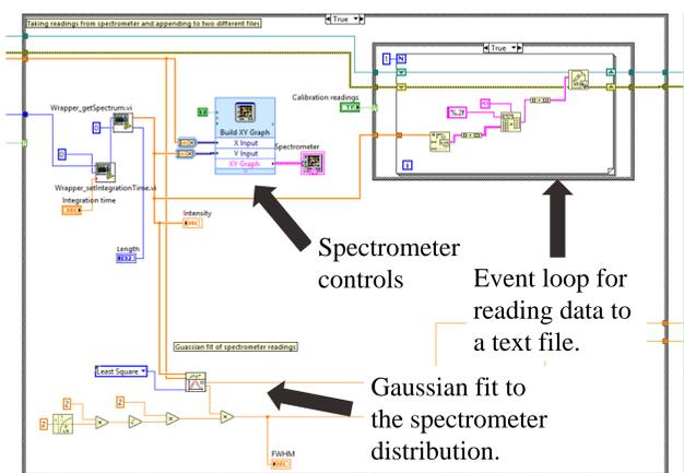
Figure 3. Event loop in the code to display and extract data from the spectrometer.
