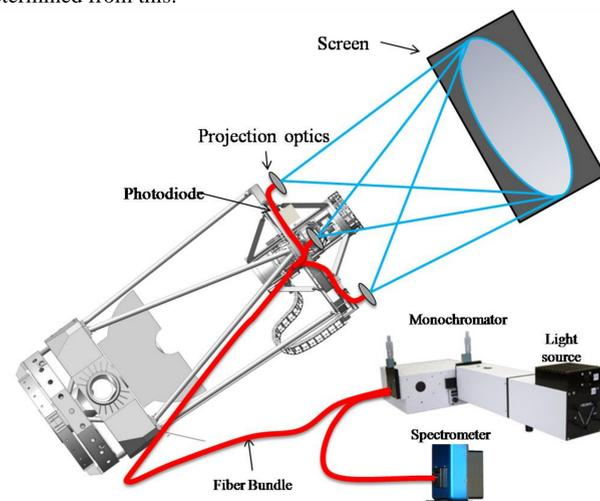
Figure 1: Astrocal and DECal set up[1]
