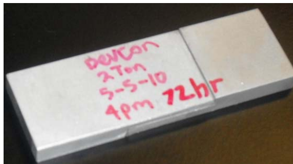
Figure 4. A fully cured epoxy sample ready for testing.
