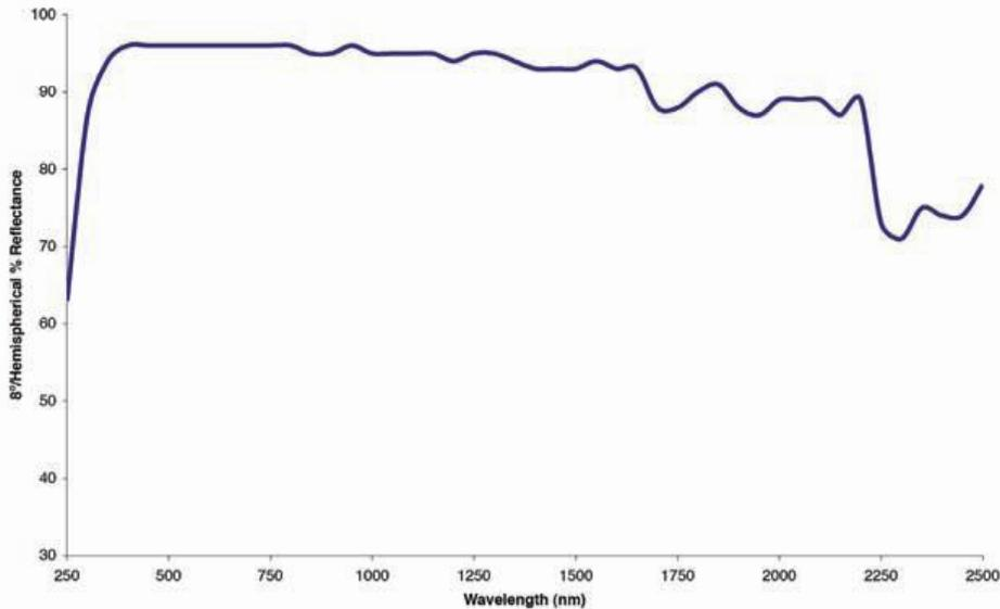
Figure 5. Duraflect reflectivity as a function of wavelength.
