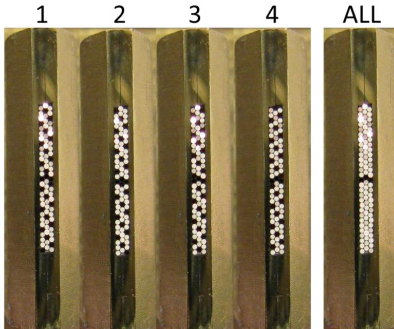
Figure 3. Fiber bundle input slit. This figure shows the mapping of the 5 output branches on the input slit. The 4 images on the left were taken while shining light in 3 out of the 4 main output fiber bundles. The 5<sup>th</sup> picture labeled “ALL” was taken with all the fiber bundles illuminated except for the wavelength sampling bundle that feeds the spectrograph.
