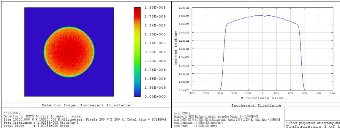
Figure 4. Left: illumination pattern from the 4 fibers projected on the flat field screen. Right: a horizontal cross-section of the light pattern.
