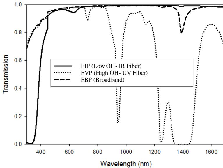
Figure 2. Internal transmission for different fiber types. All of the fibers have 10 m length.
