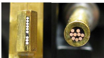
10 fiber prototype bundle used at LCO. The final bundle will consist of 87 fibers arranged in 3 vertical lines at the slit end and will be split into 5 branches at the top of the telescope.
