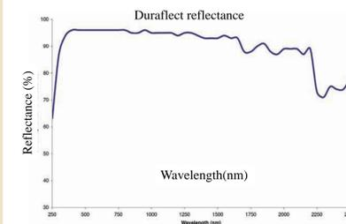
The screen we use is made of a lightweight aluminum honeycomb panel coated with a highly reflective and almost perfectly Lambertian coating called Durafluct from Labsphere. It is a coating that was developed for use in integrating spheres. The spectral reflectivity of the Durafluct coating is excellent with reflectivity over 95% from 350 to 1200nm and over 85% from 300 to 2200nm. This is shown in the figure at left.
