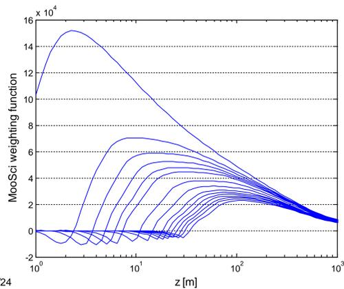
The current model incorporates into the weighting function the Moon’s phase, apparent diameter, local wind speed, and the angle of the Moon’s terminator with respect to the baseline of MooSci’s detectors. Reconstruction of the profile begins after the weighting functions and covariances of the individual baselines are calculated.
