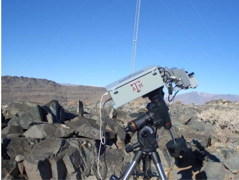
Figure 7. MooSci is shown ready for operations at Las Campanas Peak in May 2010. The initial MooSci campaign will be to profile the future site of the Giant Magellan Telescope.
