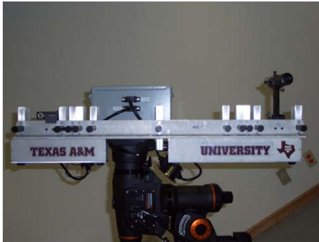
Figure 1. Given established methods for reducing data from Tokovinin’s LuSci<sup>3</sup>, MooSci has the baseline of a single LuSci mirrored around a central axis. The locations of the detectors are 0, 12, 15, 17, 21, 40, 59, 63, 65, 68, and 80cm.
